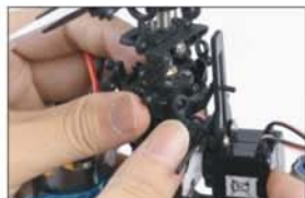
17. 将左右伺服器拉杆连上 Link up all the push-rods on the left right servos.
