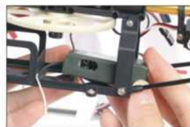
6. 将接收机放进机身并用双面胶粘好 Put the receiver into the body and stick up with double paste.
