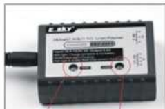
电源指示灯 Power light
